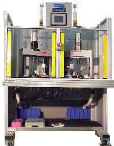
One of two ABS brake solenoid valve test stands built for Delphi Automotive Systems.
